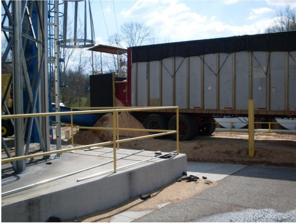
*Figure 1. Walking floor trailer offloading sawdust at the Rönile plant.*
