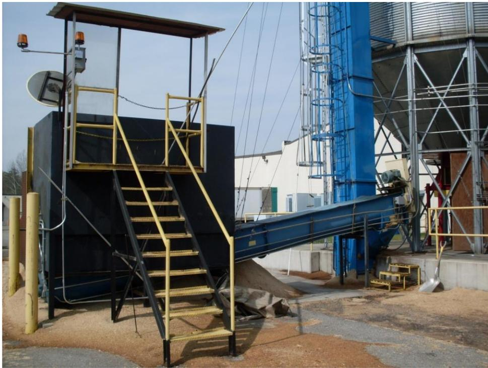
*Figure 2. Back side of Rönile's receiving bay from where the sawdust is augured into the storage silo.*
