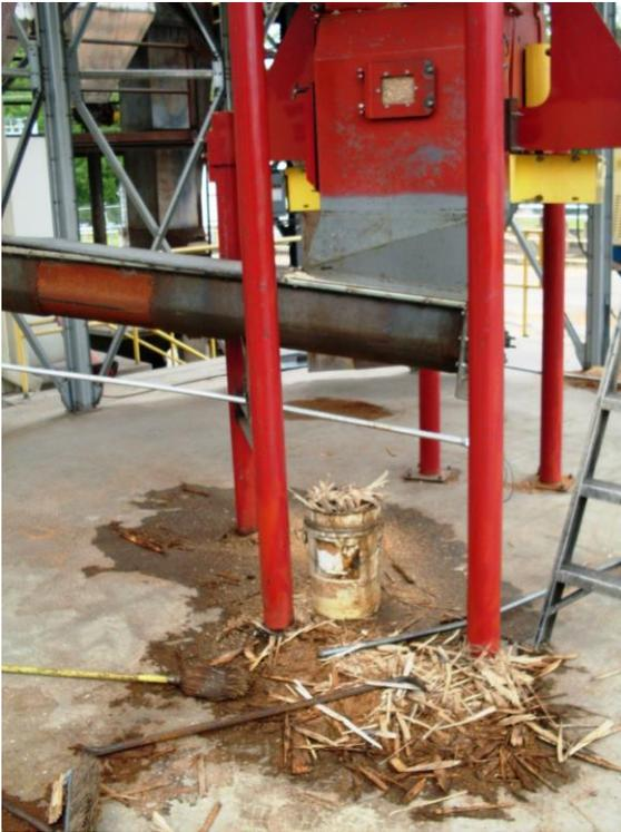
Figure 6. Example of overs (oversized material) screened out of the saw dust supply received by Rõnile.
